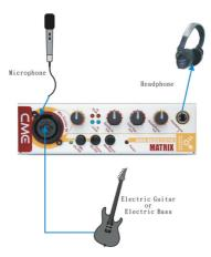
Note: You can only connect ONE device to the XLR / TS combo connector at the same time, either an XLR microphone or TS E.guitar/bass. The fig. Shows that the XLR / TS combo connector can be used to connect XLR microphones, as well as TS E.guitar/bass, but you cannot connect XLR device and TS device at the same time.
